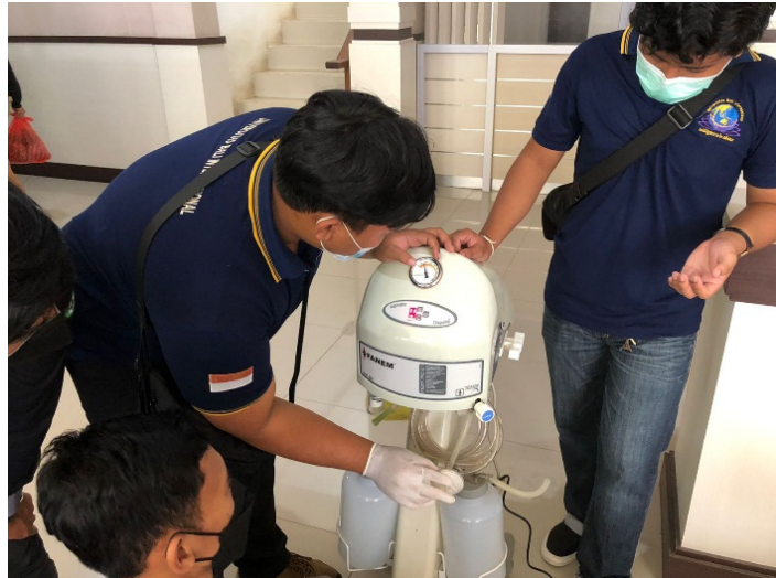
Gambar 6. Pengecekan dan penggantian filter suction pump
