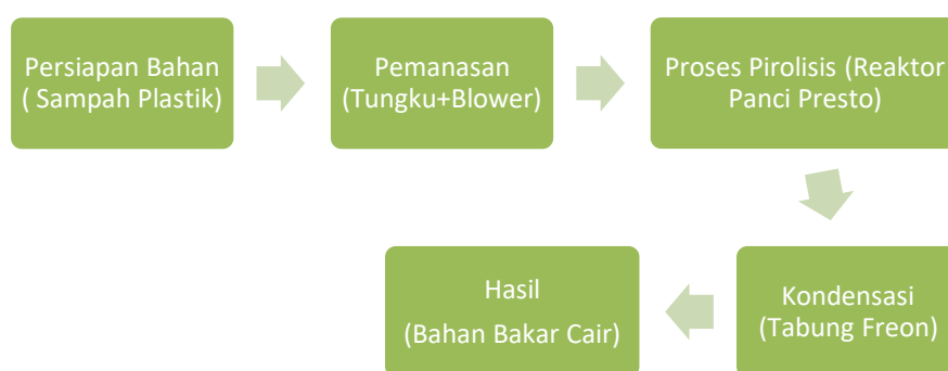
Gambar 1. Diagram alur proses pirolisis
