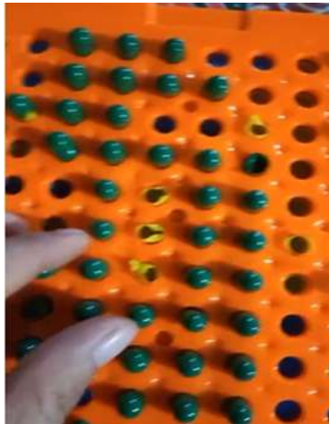
Gambar 7. Alat kapsul manual / filler capsule
