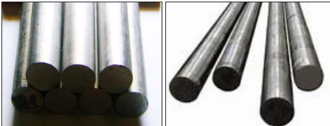
Gambar 2. Material Uji (a) Aluminium, (b) Baja Karbon
